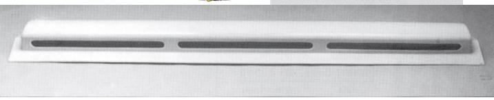
MOLDED FBERGLASS CONSTRUCTION, PROVIDES A CORROSION RESISTANT DURABLE VENTILATOR. VENT IS INSTALLED IN CONJUNCTION, WITH NORMAL RIDGE MATERIAL. SOLID MESH SCREEN PREVENTS BIRD INFILTRATION THROUGH VENTILATOR. SIMPLE GRAVITY OPERATION PROVIDES FOR EFFECTIVE, LOW COST AIR FLOW.
